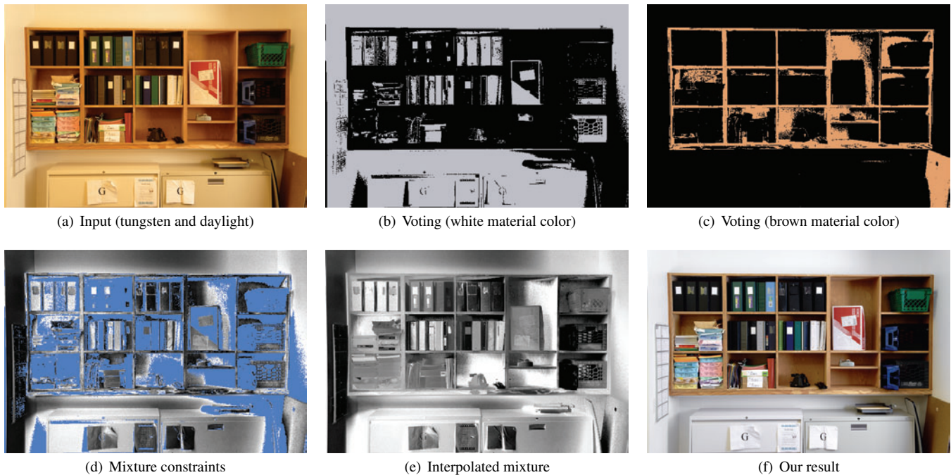
Figure 2: An overview of our approach. Given an input image (a), we extract dominant material colors using a voting technique. Here, it identifies pixels corresponding to white (b) and brown (c) material colors. This information is used to estimate the local relative contributions of each light (d). The voting scheme only labels reliable pixels. The unreliable pixels, shown in blue, are inferred using an interpolation scheme (e). The mixture information can then be used to compute a visually pleasing white balance (f).
